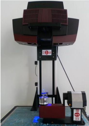
Fig. 2 – Scanning the milling tool using an optical 3D scanner GOM ATOS II TripleScan. Source: own research
